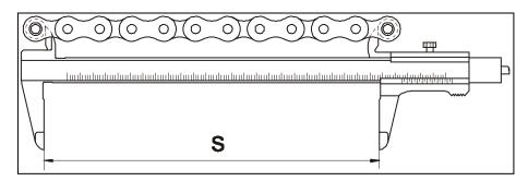
Figure 22 Wear measurement chain drive
