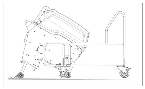
Figure 17 Moving into maintenance position
