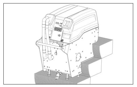
Figure 13 Insert dirty water tank
