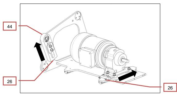
Figure 23 Tightening the chains
