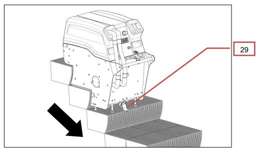
Figure 14 Removal of machine from escalator
